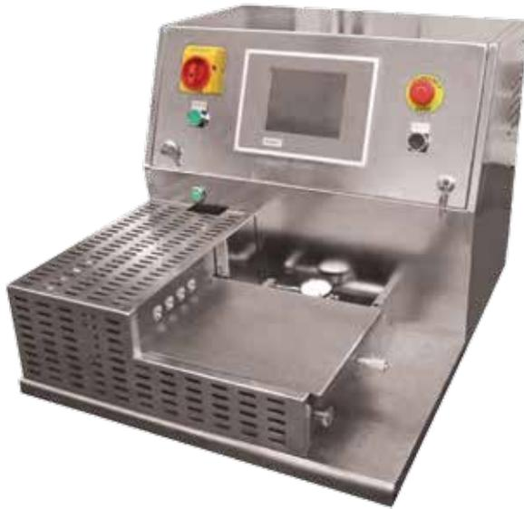
TF - 803 model was designed for non-precision applications where multiple catheters are formed simultaneously and slight tip variations are tolerable.
