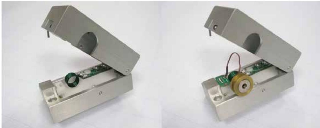
The Forming Die and Coil are mounted inside the Modular Cassette.
