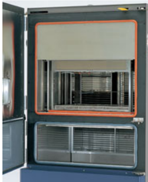
Test areas (top: high temperature chamber bottom: low temperature chamber)
