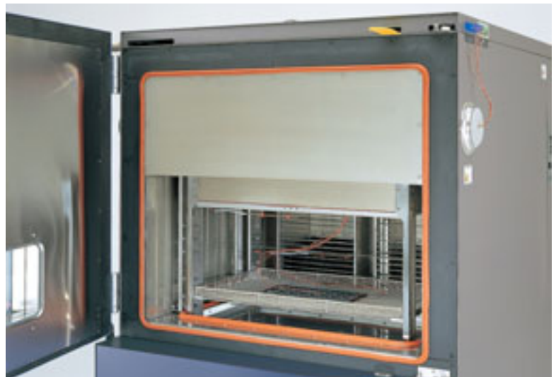
Specimen temperature measurement (specimen temperature input standard equipment: 2 locations optional: 3 locations)
