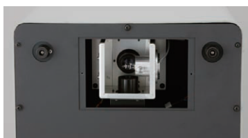
Lamp replacement area
